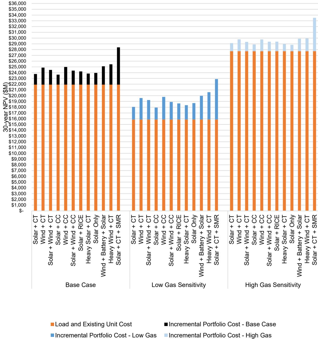
**Figure 31 – Status Quo Future Case Portfolio Cost including Load and Existing Generation Units with CO<sub>2</sub> Tax Sensitivity and Energy Evolution Scenario**
