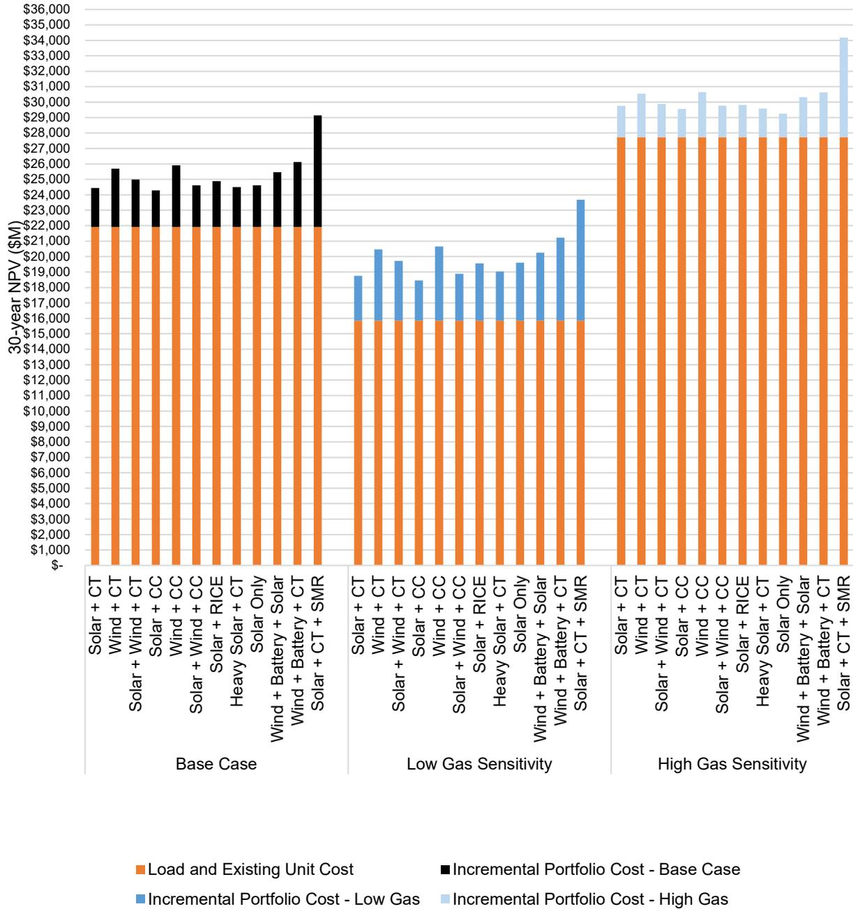
**Figure 20 – Portfolio Cost including Load and Existing Generation Units with CO<sub>2</sub> Tax Sensitivity and Energy Evolution Scenario**
