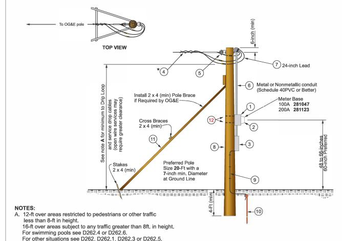
B. Use 1/2" thru bolts on top and bottom to mount meter base.
